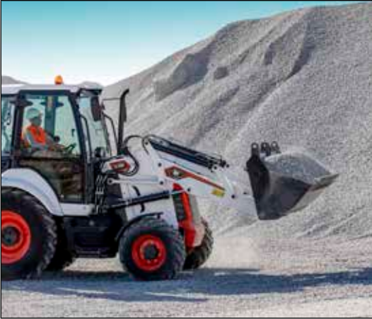
Combination Bucket: 6 in 1 Ready Piping required on the machine for operation of the bucket.
