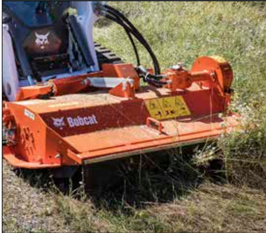
Flail Cutter: Machine must have front hydraulic auxiliary.
