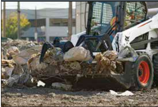
Industrial Grapple: Includes Bolt-On Cutting Edge.
