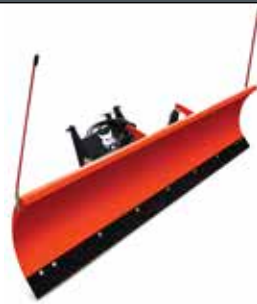
Snow Blade: Includes hydraulic angle.
