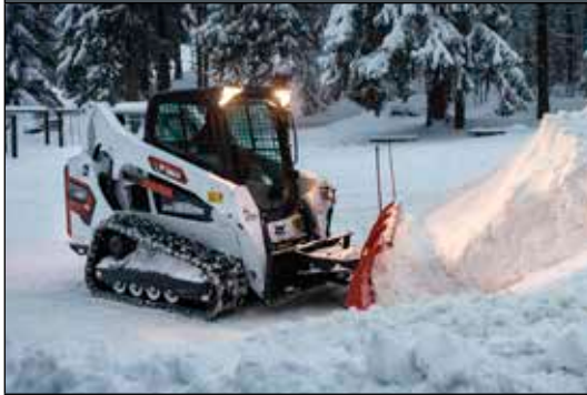
Snow Blade: Includes hydraulic angle.
